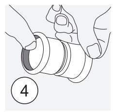
**Inspect** Fitting & Ring Seals Check that the rubber ring seal is not damaged, the correct type (colour) and both fitting & seal are free of debris.
